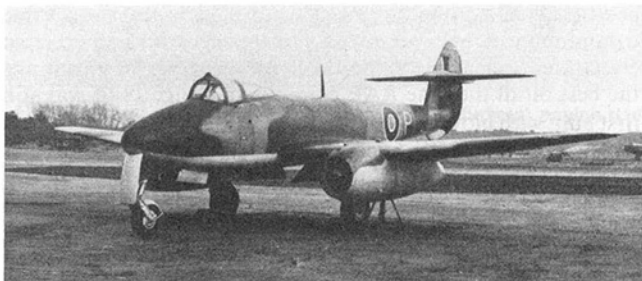
Fig. 34 Modified Gloster F9/40 with F2 engines (reprinted with permission of RAE Crown Copyright)
